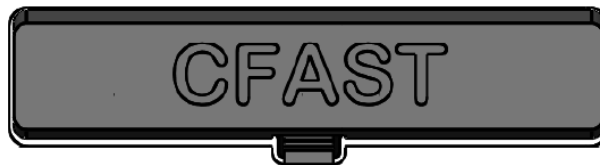
Figure 15: CFast with dust protection flap
