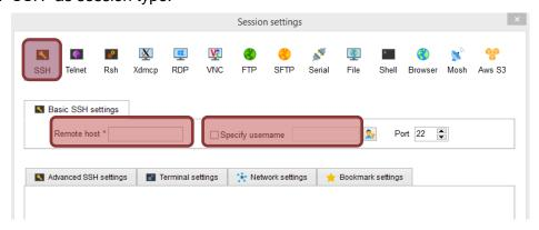
In the text field "Remote host", enter the serial number of the camera without the hyphen and add the domain ".local". You can find the serial number on the camera.
