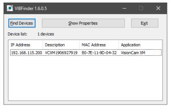
In this example, the camera has the IP address 192.168.115.200.
