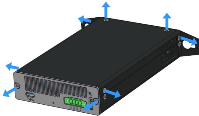
Figure 11: Remove front and top cover to access fans.
